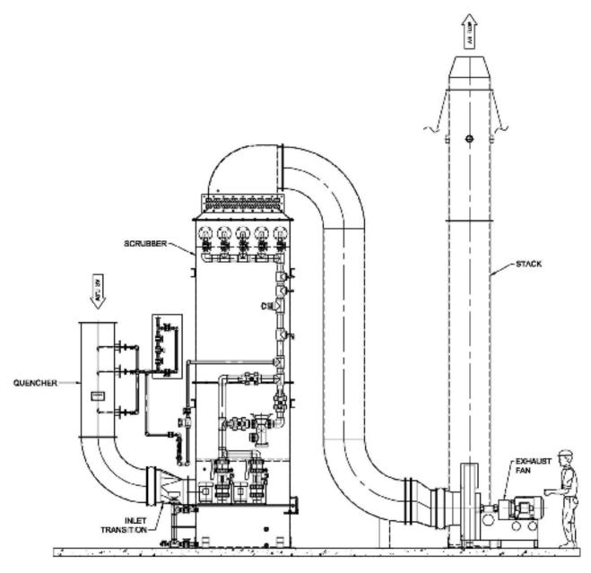
QUENCHER AND COUNTER CURRENT VERTICAL SCRUBBER SYSTEM
