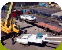
Flextor offers a complete line of heavy-duty guillotine dampers to meet your requirements. We have installed dampers in ducting sizes as large as 25' high by 16' wide. Our zero-leakage designs have been hydrotested as high as 3 PSI and hydro tested at 60 PSI for structural integrity.
