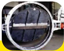
Flextor offers a complete line of heavy-duty butterfly dampers to meet your requirements. We have installed butterfly dampers as small as 2" diameter, to as large as 120" diameters and more. Our butterfly dampers can be found in some of the harshest environments where abrasion, corrosion and dust-loading are prevalent.
