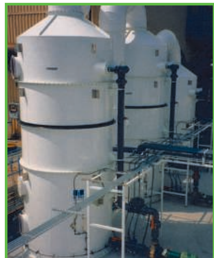
Application: Oxidation/Reduction of NO x Problem: Total NO x = NO + NO 2 Solution: Beta Nox 2000® Three Stage
