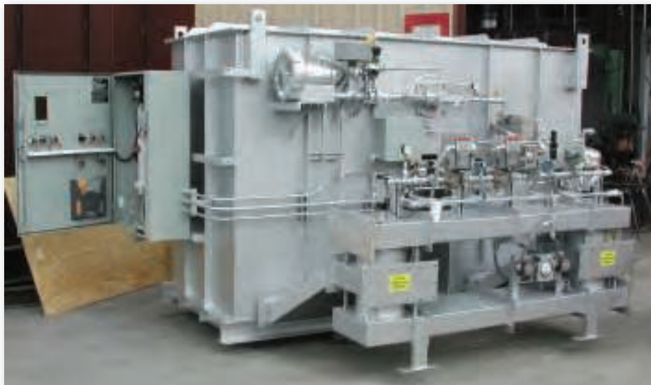
Skid mounted Retox RTO for halogenated chemical VOCs.
