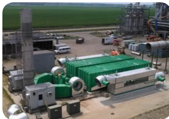
RTO 处理乙醇干燥和生物燃料尾气 RTO for Ethanol Drying and Biofuels
